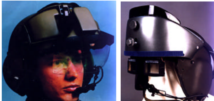
Figure 12: Two optical see-through HMDs, made by Hughes Electronics
